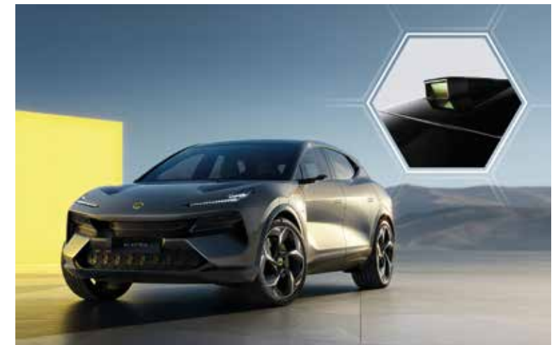
Automated driving (Level 2-3): The world's first retractable Roof Sensor Module integrates lidar and sensor redundancy systems on the roof for improved aerodynamics and aesthetics.
