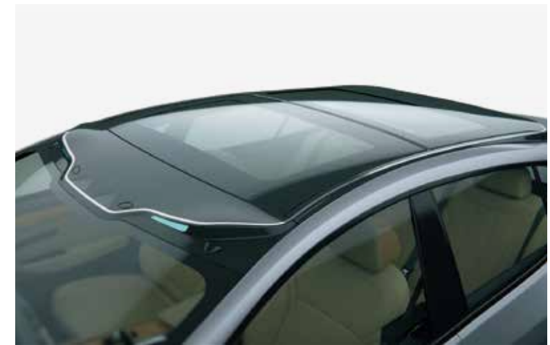
Autonomous driving (Level 3-4): A total of 14 sensors are integrated in a slim, elegant panoramic roof to enable autonomous driving.
