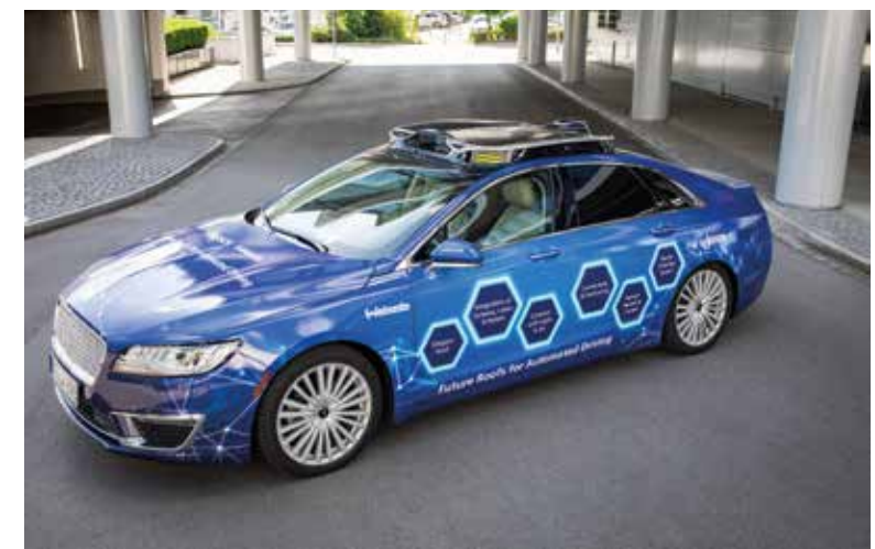
Fully autonomous driving (Level 4): Four radar, four lidar and 16 camera sensors of different types from Bosch are integrated in this Roof Sensor Module.
